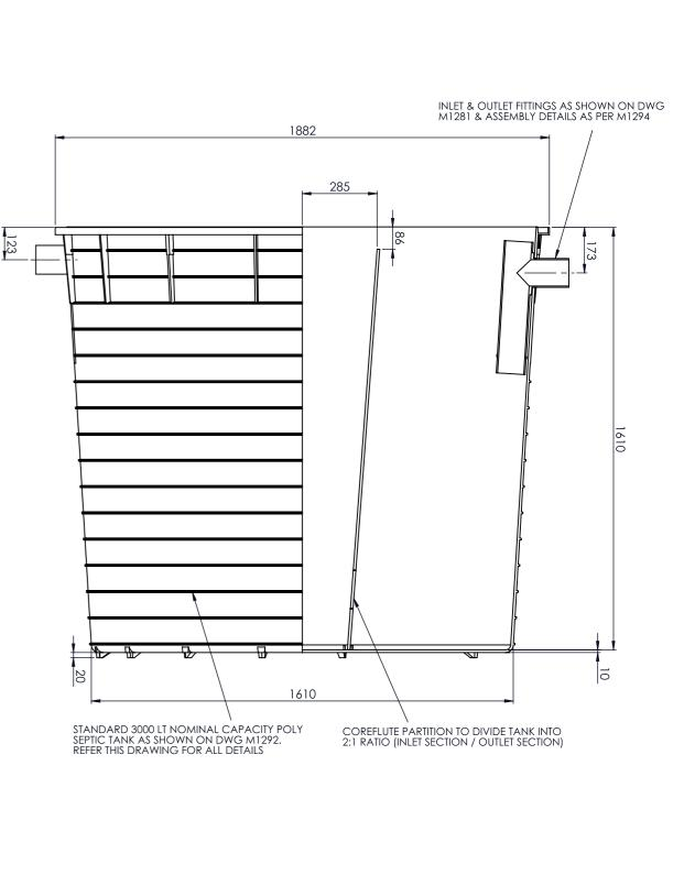
\*Drawing does not include the lid of the septic tank
